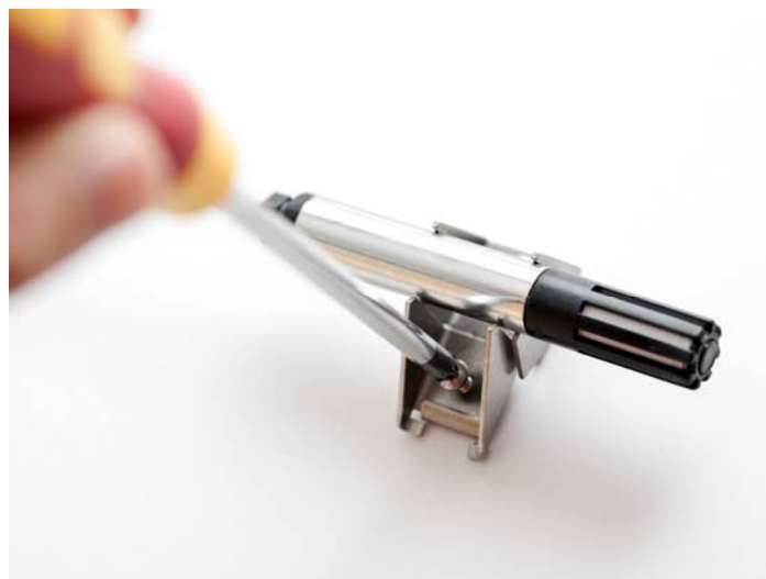
Figure 10 Tightening the Lower Clamp Part
