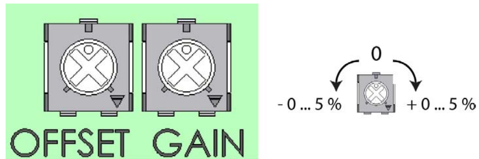
Figure 17 Trimmers for Offset and Gain
