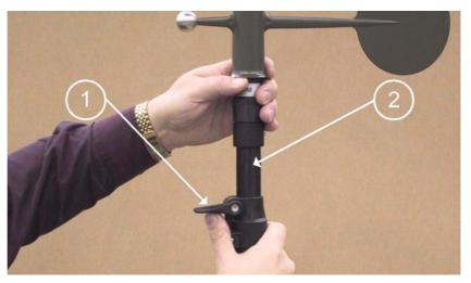
Figure 37 Extending the Telescopic Mast
