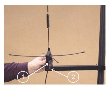
Figure 41 Installing UHF Antenna to Arm
