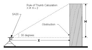
Figure 27 SA20M Vertical Obstruction (Side View)
