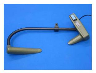
Figure 19 Present Weather Detector PWD22M
