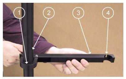
Figure 39 Installing UHF Antenna Arm
