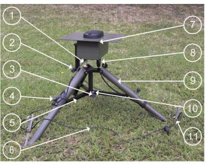
Figure 59 Lightning Detector SA20M with Grounding Net
