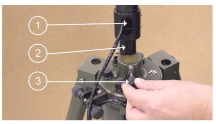
Figure 36 Attaching the Telescopic Mast
