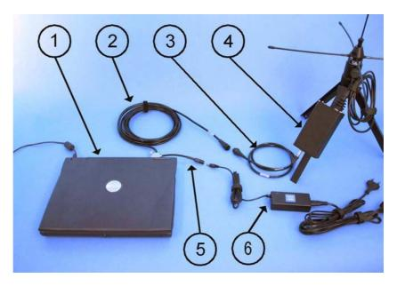
Figure 48 Connecting the Radio Modem to PC
