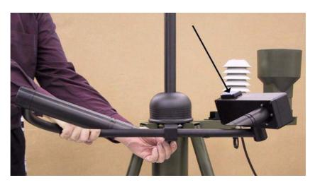
Figure 55 Installing PWD22M (Arrow Pointing to Rain Detector Plate)
