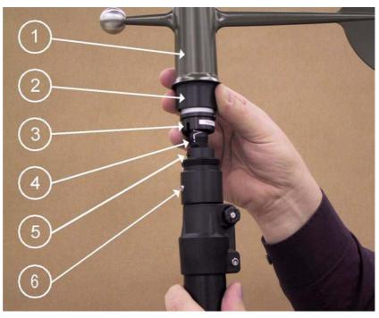
Figure 35 Wind Sensor Attachment
