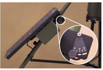
Figure 47Setting the Correct Tilt Angle
