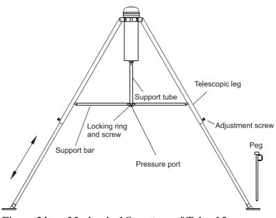
Figure 34 Mechanical Structure of Tripod Legs
