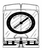
Figure 25 Sighting Line of the Mirror Runs in the Middle of the Capsule View
