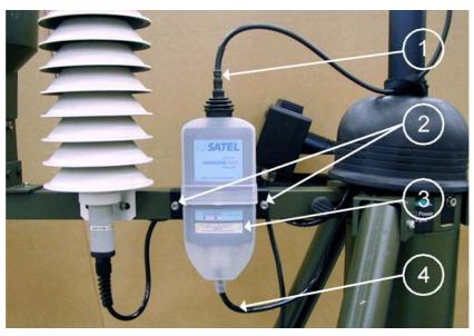
Figure 42 Installing Radio Modem
