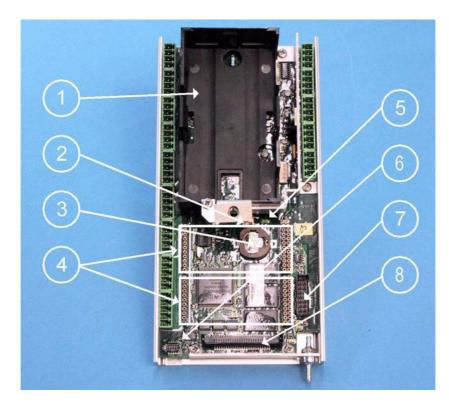
Figure 6 AWS Logger QML201 without Cover
