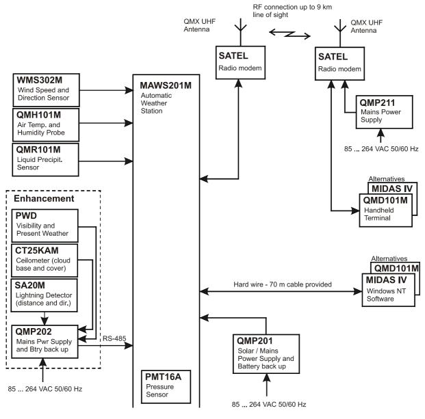
Figure 1 Block Diagram of the Basic System and Enhancement
