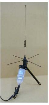
Figure 49 UHF Antenna on Tripod
