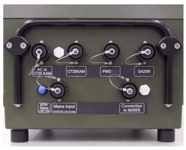
Figure 54 Connectors on the Mains Power Supply QMP202
