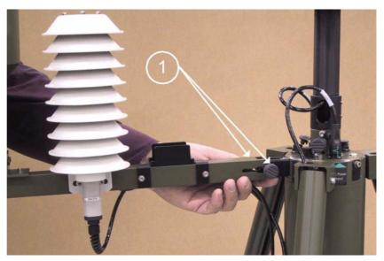
Figure 38 Sensor Arm Attachment
