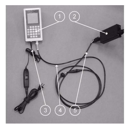
Figure 50 Connecting Radio Modem to the Handheld Terminal
